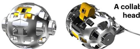
A collaboration between the Japan Aerospace Exploration Agency (JAXA) and Tokyo-headquartered toy-maker TOMY, has produced a baseball-sized robot to explore the moon surface. The toy company's expertise in small, moveable parts helped produce this ultra-lightweight robot that can hitch a ride on the lunar lander. The bot can easily roam the uneven surface of the moon and also has a camera to capture photos.
