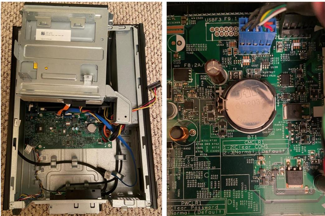
Figure 1: Computer opened after removing five screws and disengaging eight metal tabs and three plastic tabs (left); close-up of coin cell battery (right)
